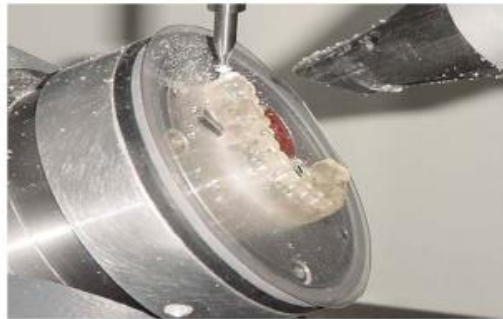
Figure 2. aligner models are created using stereolithography and CAM
