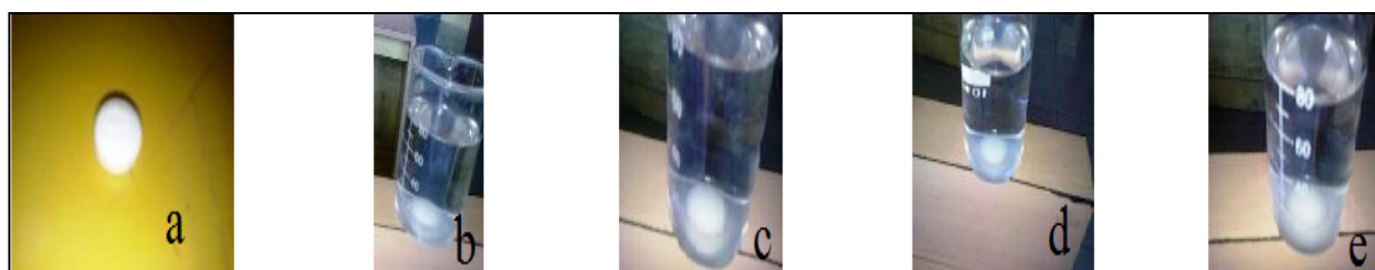
Figure 6. Homogeneous core tablet (a), after one hour (b), after three hours (c), after five hours (d) and after eight hours (e)
