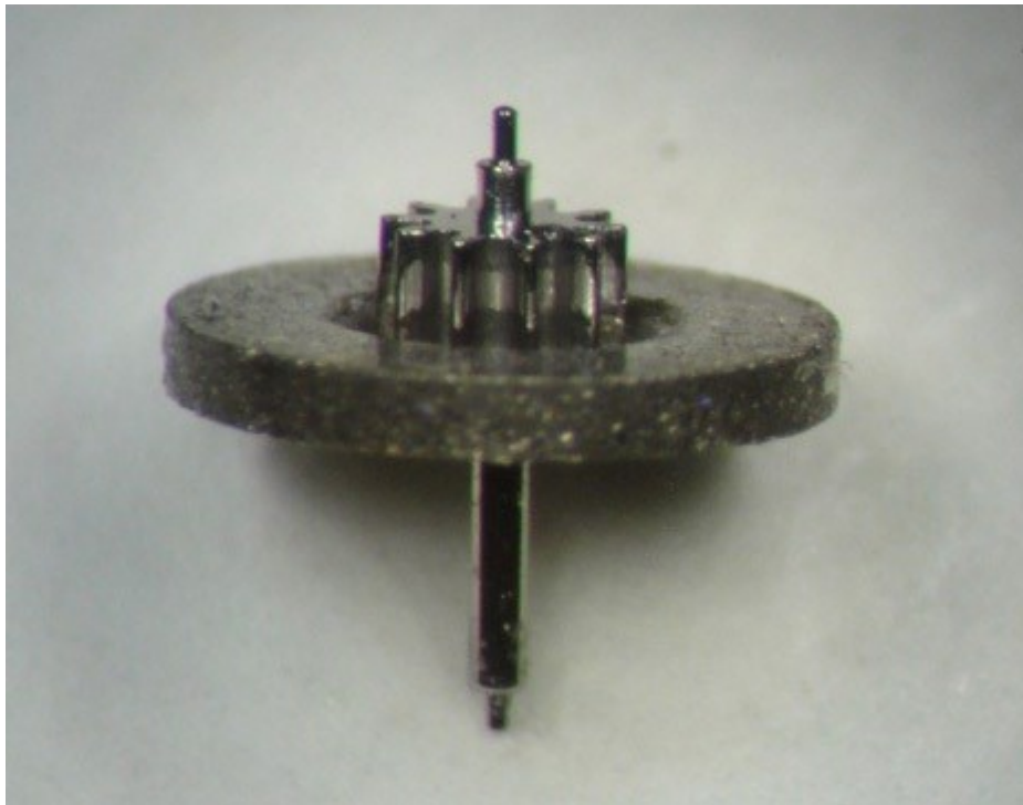
Fig. 1. A turbine in an artery could harvest enough energy from blood flow to power implanted medical devices. Image credit: Alois Pfenniger, ARTORG Cardiovascular Engineering, University of Bern, Switzerland
