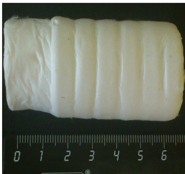
Figure 1: Sample of tracheal matrix based on polymeric ultrafibrous materials for experiments on dogs
